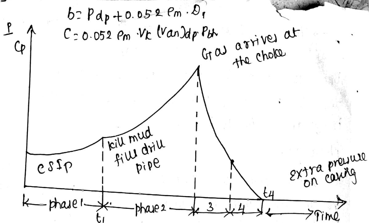
Engineering method - Casing pressure vs. time.
