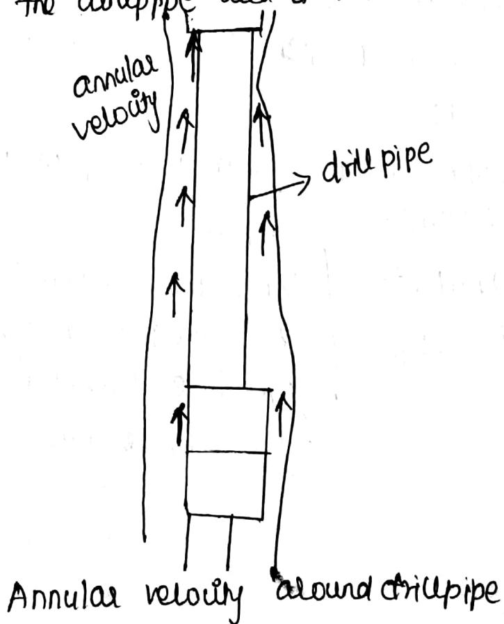
Annular velocity around drill pipe
