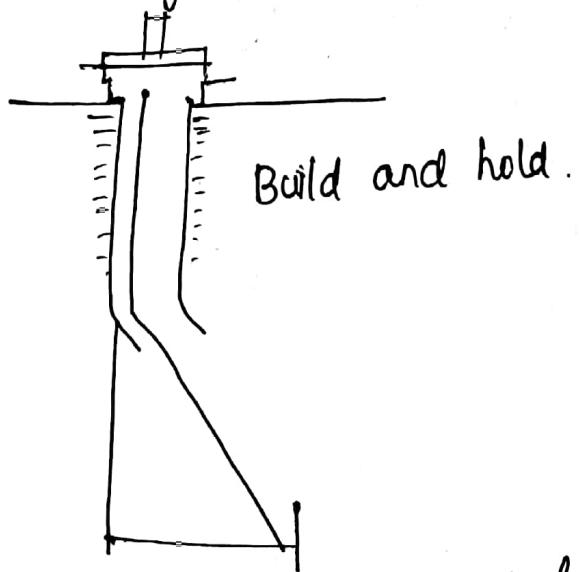
→ These profiles can be used for moderate-depth drilling in areas where intermediate casing is not required and where oil-bearing strata are a single horizon.
