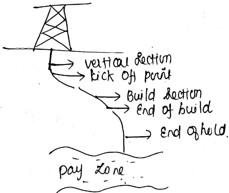
→ Type II wells are made up of a vertical section, a kick-off point, a buildup section, a tangent section, a drop-off section and a hold section upto targets.
