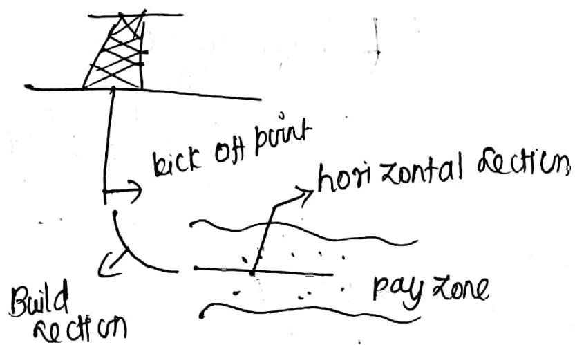
→ Type III wells are made up of anyone of the above profiles plus a horizontal section within the reservoir. They are also called horizontal wells or horizontal directional wells.
