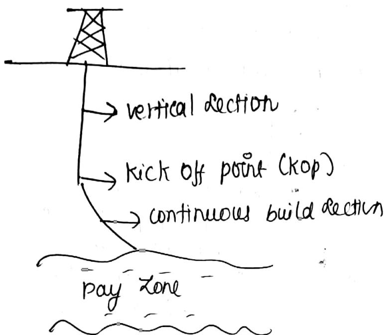
→ Type II wells are made up of a vertical section, a deep kick off and a build up to a target.
